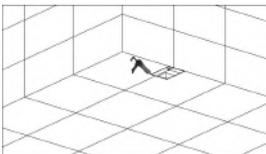
10. Filled silicone between floor drain and ceramic
