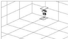
11. Install the odor protection box and cover the filter net
